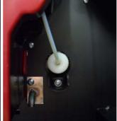
4. Reconnect the brewer inlet pipe using the knurled thumbwheel.
