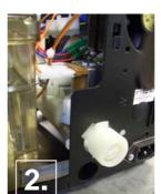
2. This figure shows the correct assembled position for the mains inlet valve.
