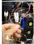
4. Reconnect the connections of the tank inlet valve to the extension cables of the mains inlet valve.
