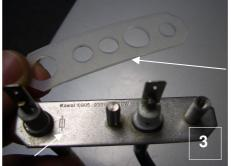
3. The new element has internal thermal protection (identifiable by Symbol shown). Ensure that the rubber gasket is fitted the correct way.
