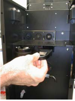
remove the pipes support; remove the mixing bowls, the mixing fan. and the aspiration drawers.
