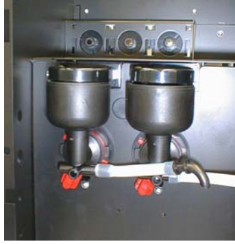
remove the pipes support; remove the mixing bowls, the mixing fan. and the aspiration drawers.
