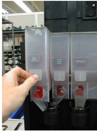
Remove all the ingredients canisters from the machine and disassemble
