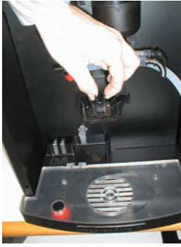
remove the pipes support; remove the mixing bowls, the mixing fan. and the aspiration drawers.
