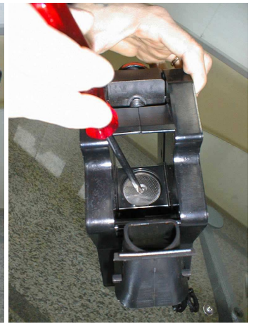
Dismount the inferior filter and clean it with hot water removing all coffee powder. Reassemble the group in the original position.
