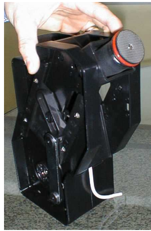
Turn upwards the superior filter, dismount and clean it with hot water removing all coffee powder.
