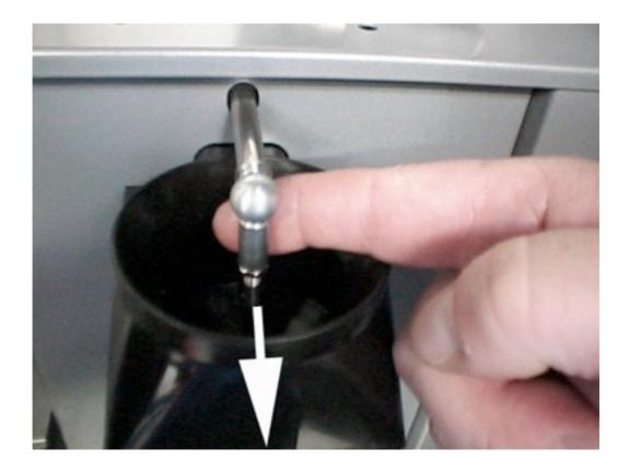
(11) Move the upper locking lever (C) to the vertical, (unlocked position) and remove the brew chamber assembly (D) by pulling it gently towards the front of the machine.
