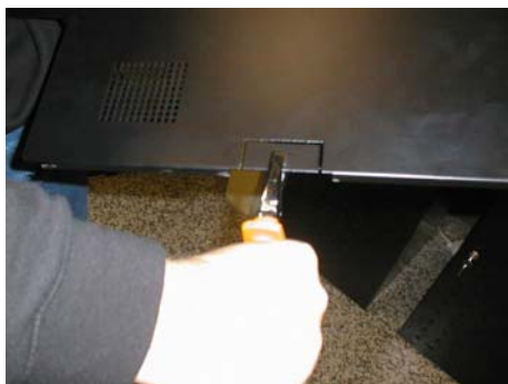
Cut the rear wall to make a hole for Damian Piccola to connect the communication cable. Install again the rear wall of the XM vending machine.
