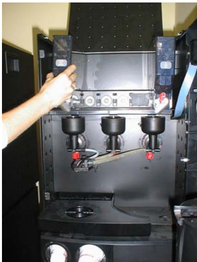
Remove all the ingredients canisters from the machine and disassemble completely the canisters
