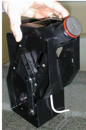
Turn upwards the superior filter, dismount and clean it with hot water removing all coffee powder.
