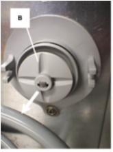
(13)Remove the impellor disk **B** by pulling it in the direction shown.
